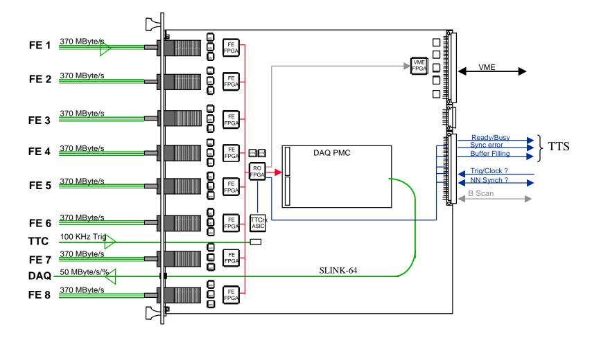
will be on a transition module mounted on the rear of the backplane. Figure 1: A somewhat out-of-date design of final FED. We now envisage that the SLINK driver
