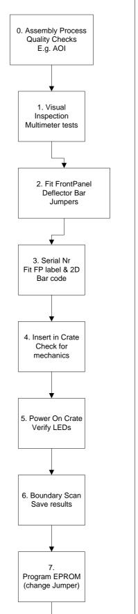
For details of tests and checks and acceptance criteria see detailed diagrams
