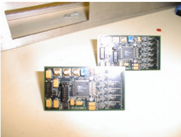
Figure 5: The cross-point switch based electrical test cards.
